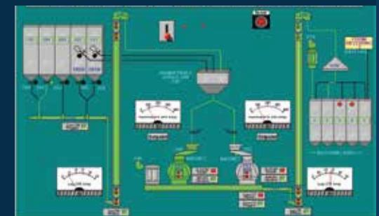
Automation Systems have control modules designed for any size Receiving, Grinding, Flaking, Batching, Pelleting, Coating, and Load Out requirements.
